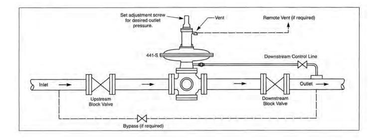
**Periodic Inspection:** Regulators are pressure control devices with numerous moving parts subject to wear that is dependent upon particular operating conditions. To assure continuous satisfactory operation, a periodic inspection schedule must be adhered to with the frequency of inspection determined by the severity of service and applicable laws and regulations. **See Bulletin RM-1350 for field service instructions.**
