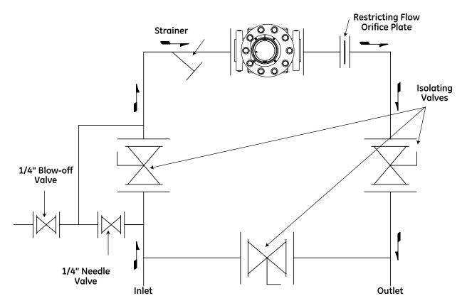
Figure 3 -Side Inlet Configuration for Series B3 HPC Meter
