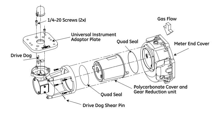
Figure 14 - Assembly Instrument Drive to meter end cover
