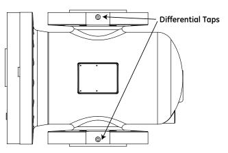
$\ensuremath{\mbox{Figure 16}}$  - Differential pressure taps are located above and below the meter nameplate
