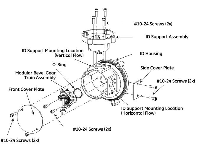
Figure 13 - Exploded View of Instrument Drive (ID) Assembly
