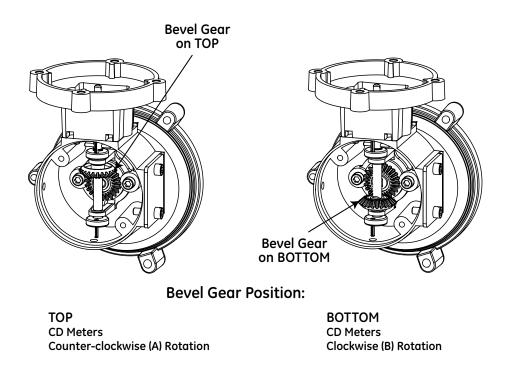
Figure 14 - Placement of bevel gears determines rotational direction
