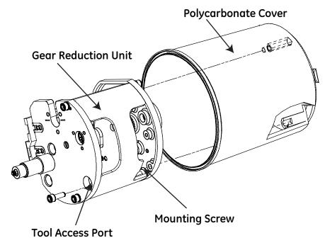
Figure 12 - Exploded view of Gear Reduction Assembly and Polycarbonate Cover
