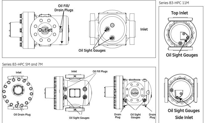
Figure 6 - Oil fill/drain plugs and oil level sight gauge locations
