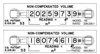
Figure 9 - Non-Compensated Series 3 Metric Unit odometers for 1M (Top), 5M (Bottom)
